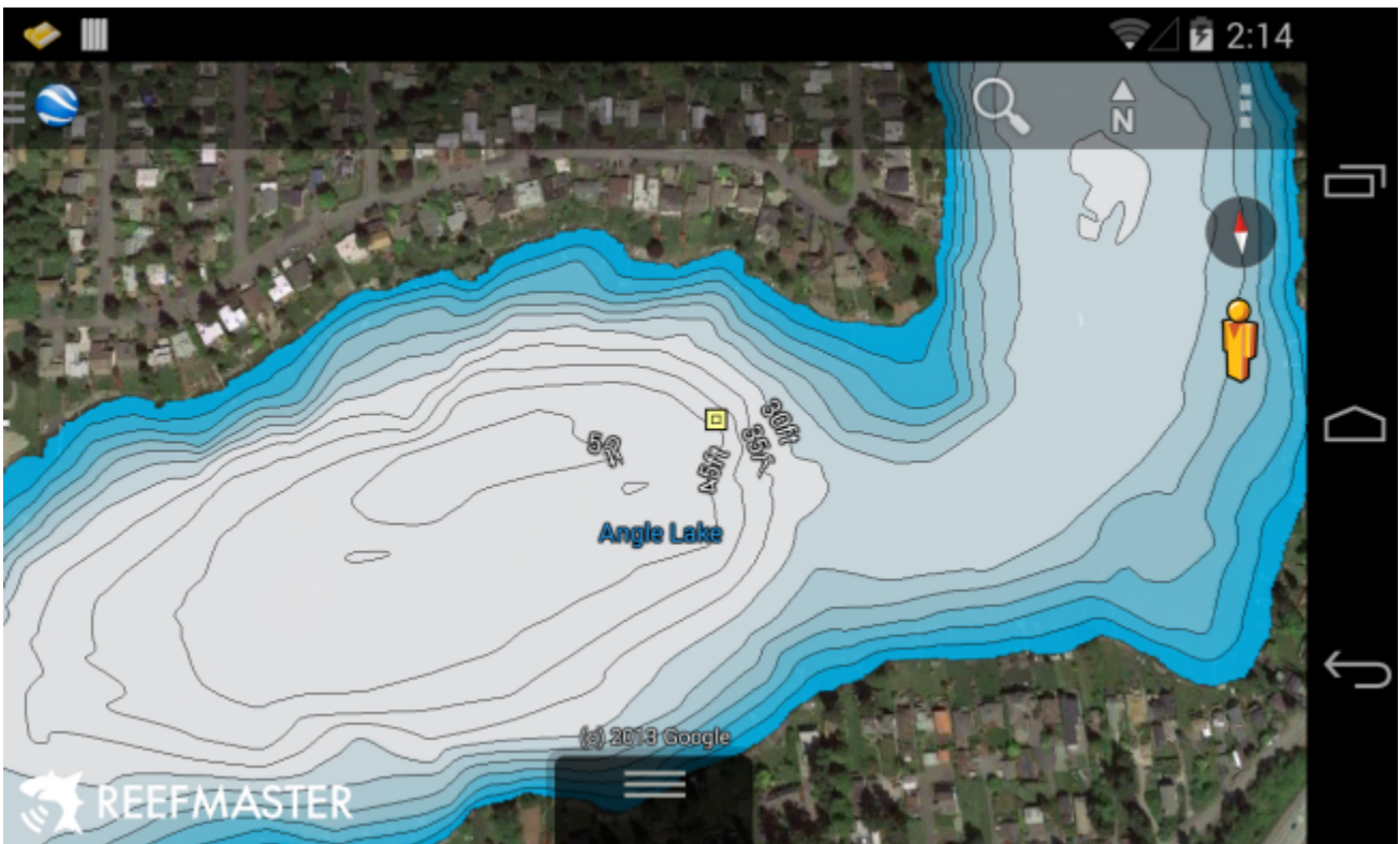
Lake contours as viewed on the Google Earth mobile application, running on a Google Nexus 4 smart phone. The contour interval is 5 ft.
